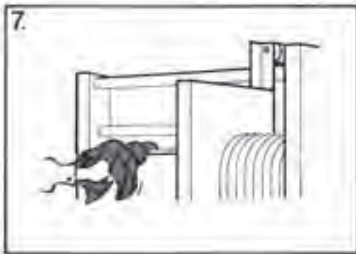
7. Inspect the sliding surfaces of the carrying bar and wipe clean
